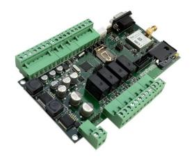
The 4CWireless – Extended Series is a feature-rich card for advance telemetry and supervisory control applications.
